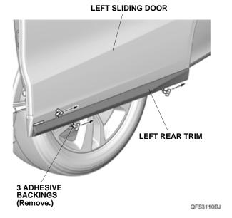
Secure the left rear trim to the left sliding door with two clips.
