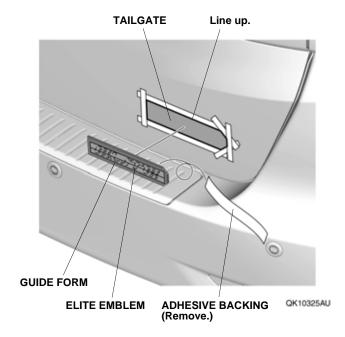
29. Remove the guide form and using the palm of your hand, firmly press the ELITE emblem against the tailgate.
