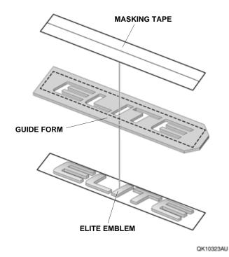
27. Using an alcohol wipe, thoroughly clean the tailgate where the ELITE emblem will attach.
