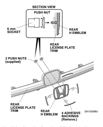
Using the palm of your hand, firmly press the rear H emblem against the rear license plate trim. 11. Remove the position film from the ODYSSEY emblem, then remove the ODYSSEY emblem from the guide form.
