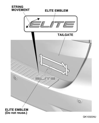
26. Install the ELITE emblem in the guide form, and temporarily secure it with masking tape.
