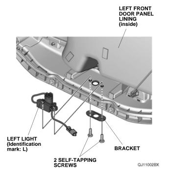
13. Secure the left light 2-pin connector to the rib on the left front door panel lining with one wire tie with clip as shown.
