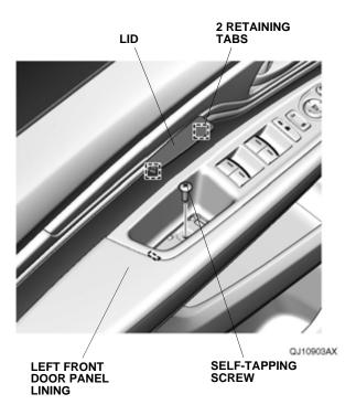
5. Remove the left front door panel lining, and unplug the vehicle connectors.
