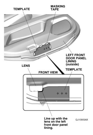
8. Using a pushpin, pierce the center of the three printed marks on the template. Remove the template.
