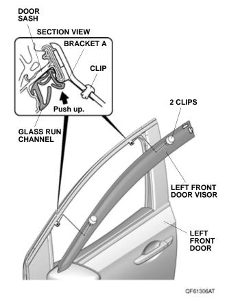
9. Secure the left front door visor to two brackets A with two clips. Make sure to push up on the two brackets A while installing the two clips.
