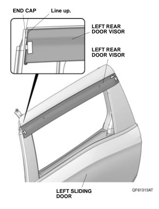
22. While applying light pressure against the left rear door visor, carefully remove the taped adhesive backings. Make sure to push up on the two brackets B while removing the adhesive backings. NOTE: While removing the long top piece of adhesive backing, make sure that the left rear door visor is positioned so that top edge of door molding is hidden by the door visor.
