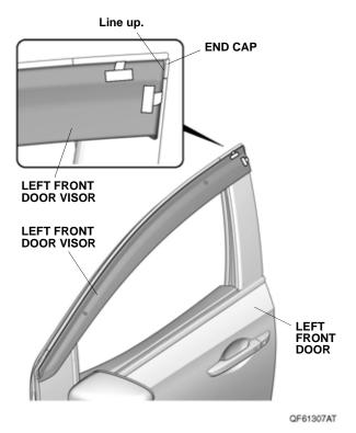
11. While applying light pressure against the left front door visor, carefully remove the taped adhesive backings. Make sure to push up on the two brackets A while removing the adhesive backings. NOTE: While removing the long top piece of adhesive backing, make sure that the left front door visor is positioned so that top edge of door molding is hidden by the door visor.
