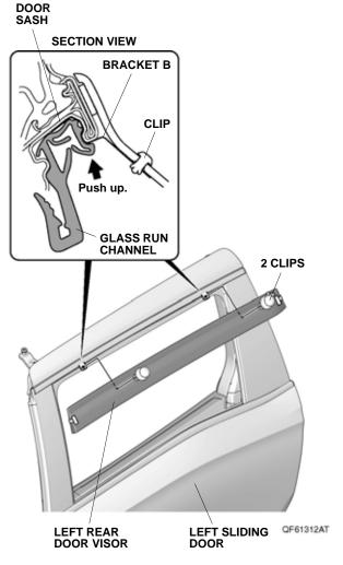
20. Secure the left rear door visor to two brackets B with two clips. Make sure to push up on the two brackets B while installing the two clips.
