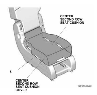
17. Secure the center second row seat cushion cover to the center second row seat cushion with one fastener.
