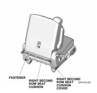
Pull down the armrests (if equipped). Fit the right second row seat-back cover onto the right second row seat-back through the seat belt. Insert the right second row seat-back cover under each headrest guide.
