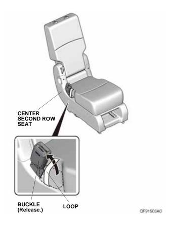
15. Fit the center second row seat cushion cover onto the center second row seat cushion.
