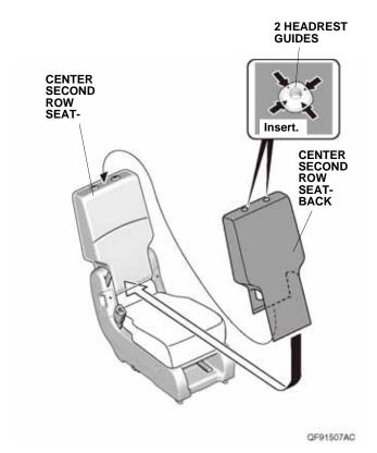
Pull down the center second row seat-back. Secure the center second row seat-back cover with one fastener.
