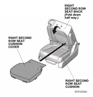
4. Secure the right second row seat cushion cover to the right second row seat cushion with the four tabs and two fasteners.
