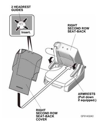
Secure the right second row seat-back cover with two fasteners.
