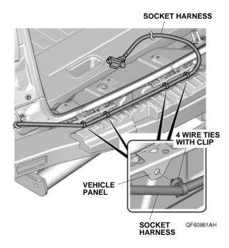
27. Route the socket harness behind the trailer hitch as shown.
