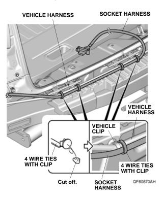
25. Secure the socket harness to the vehicle harness with four wire ties with clip. Go to step 27.
