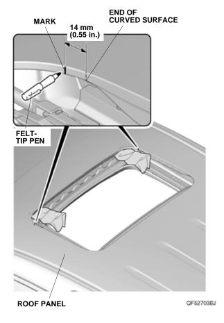
4. Using an alcohol swab, thoroughly clean the roof panel at each of the two marks you have made but do not wipe off the mark.
