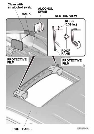
5. Remove the adhesive backing from the two protective films and attach one to the roof panel at each of the two marks you made. Wrap 10 mm (0.39 in.) of protective film around the lip of the moonroof opening.
