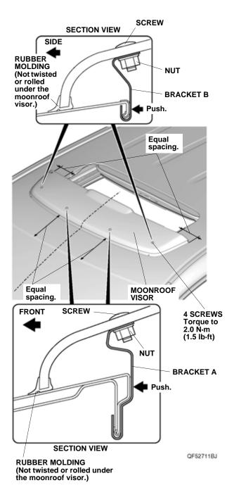
14. Tighten two screws and two nuts on the front of the vehicle first, then tighten two screws and two nuts on each side. Tighten while applying pressure so that there is no gap between the roof panel and the brackets A and B. Torque the screws to 2.0 N·m (1.5 lb·ft).
