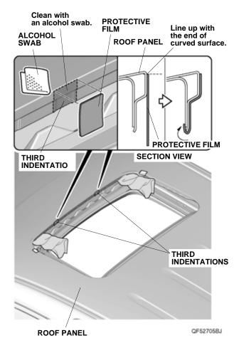
7. Remove the adhesive backing from the two protective films and attach one to the roof panel at each third indentation.
