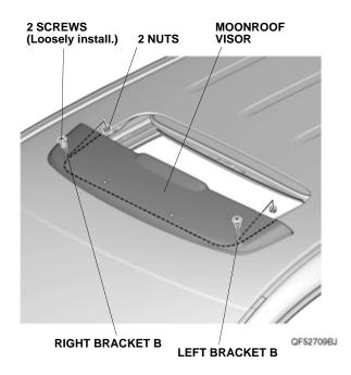
12. Check the information on the IMPORTANT INFORMATION label. To avoid wind noise, install the brackets against the body.
