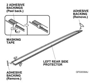
12. Line up the left rear side protector with template A and template B, and install the left rear side protector on the left sliding door.
