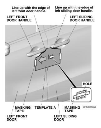
2. Line up template B with the edge of the left sliding door, making sure the arrow hole points to the rear of the vehicle. Then, attach template A to the left sliding door with masking tape as shown.
