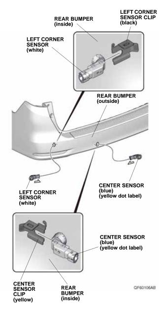
39. Secure the left corner sensor (white) and center sensor (blue) with the left corner sensor clip (black) and center sensor clip (yellow) as shown.
