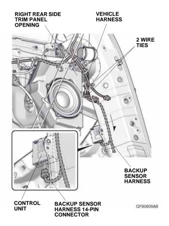
27. Secure the backup sensor harness to the vehicle harness with two wire ties.
