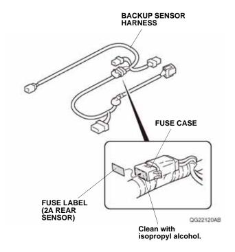
22. Remove the tape to free the vehicle 2-pin connector. Plug the vehicle 2-pin connector into the backup sensor harness 2-pin connector, and secure the 2-pin connectors to the vehicle harness with one wire tie.
