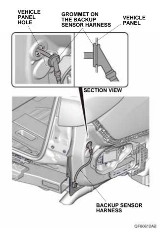
32. Install the connector clip on the backup sensor harness 8-pin connector, and secure the backup sensor harness 8-pin connector to the vehicle panel.
