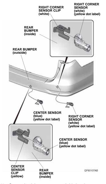
41. Secure the right corner sensor (white) and center sensor (blue) with the right corner sensor clip (white) and center sensor clip (yellow) as shown.
