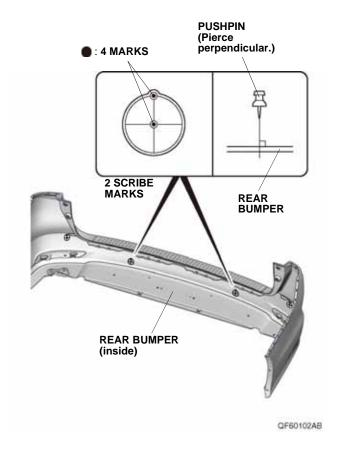
35. While wearing eye protection, drill the eight pierced marks with a 3 mm drill bit from the painted side of the rear bumper.
