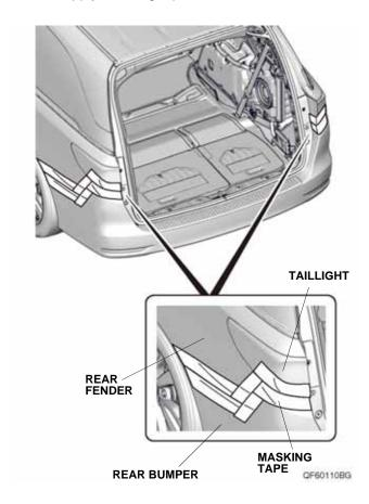
Remove the six self-tapping screws, six clips, two large hex bolts, and two small hex bolts as shown.
