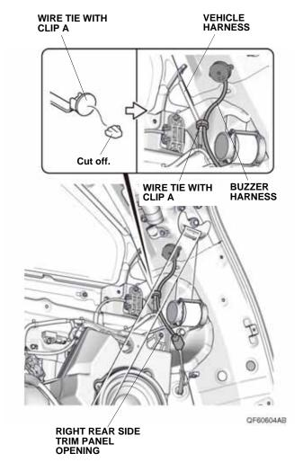
19. Secure the buzzer harness to the vehicle harness with that wire tie. Go to step 21.
