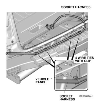
Route the socket harness behind the trailer hitch as shown.
