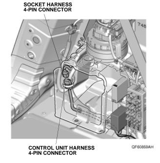
23. Secure the socket harness to the vehicle harness with three wire ties.
