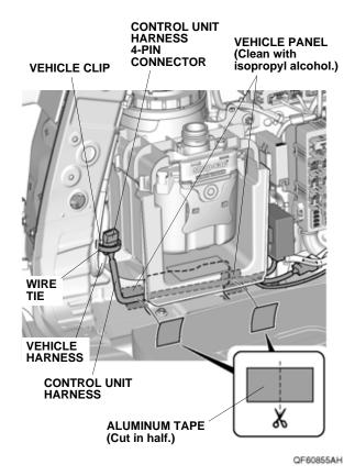
15. Using isopropyl alcohol on a shop towel, thoroughly clean the vehicle panel where the aluminum tape will attach. Using scissors, cut one aluminum tape in half. Secure the control unit harness to the vehicle panel with the two halves of aluminum tape. Go to step 18.
