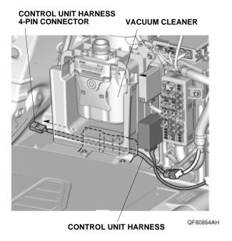
14. Line up the control unit harness 4-pin connector with the vehicle clip and secure the control unit harness 4-pin connector to the vehicle harness with one wire tie.
