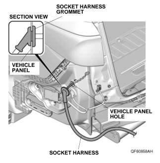
22. Plug the socket harness 4-pin connector into the control unit harness 4-pin connector.
