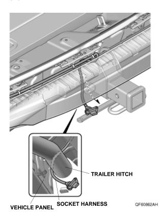
28. Secure the socket harness 4-pin connector to the trailer hitch with two flange bolts.
