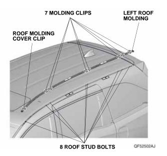
3. Using needle nose pliers, remove the seven molding clips and the roof molding cover clip from either the molding or the roof stud bolts.
