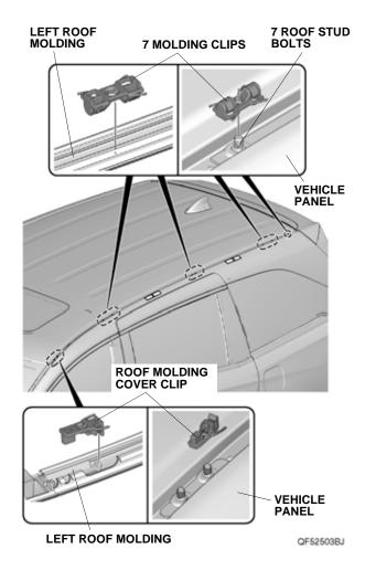
4. Using a putty knife, remove any excess sealant from the roof stud bolts.
