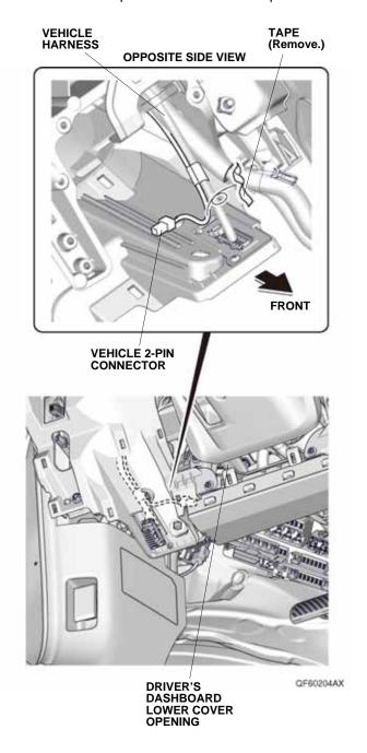
5. Install the ambient light on the instrument panel as shown.
