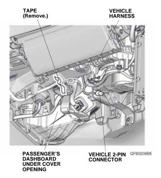
Plug the vehicle 2-pin connector into the ambient light, then install the passenger's dashboard under cover.
