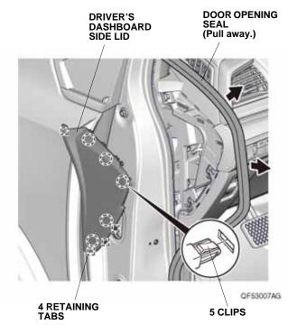
3. Remove the driver's dashboard lower cover, and unplug the vehicle connectors.
