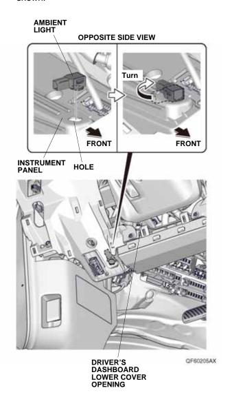
6. Plug the vehicle 2-pin connector into the ambient light.
