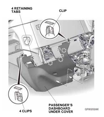
8. Install the ambient light on the passenger's dashboard under cover as shown.
