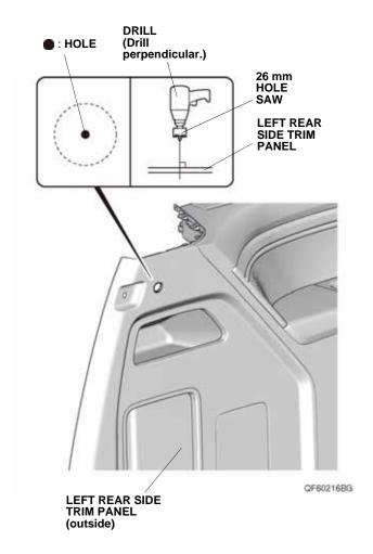
21. Install the switch into the 26 mm hole in the left rear side trim panel.
