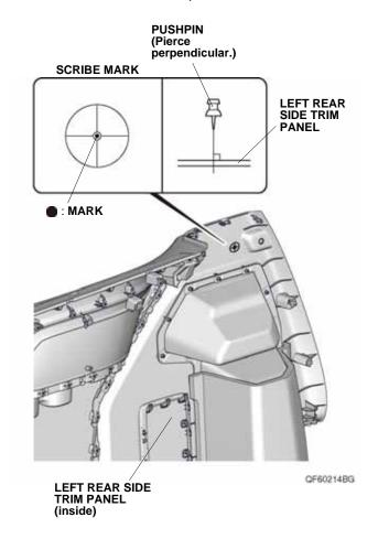
19. While wearing eye protection, drill the pierced mark on the left rear side trim panel with a 3 mm drill bit. NOTE: Make sure to drill perpendicular to the left rear side trim panel.
