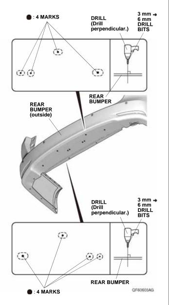
32. While wearing eye protection and drilling from outside of the rear bumper, enlarge four 6 mm holes, with a 9 mm drill bit, then finish with an 11 mm drill bit
