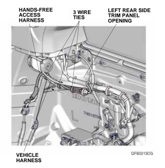
18. Using a pushpin, pierce the center of the scribe mark on the left rear side trim panel.
