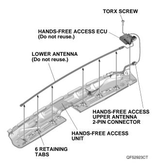
27. Install the new Hands-Free Access ECU on the Hands-Free Access unit with the TORX screw, and plug the Hands-Free Access upper antenna 2-pin connector into the new Hands-Free Access ECU.
