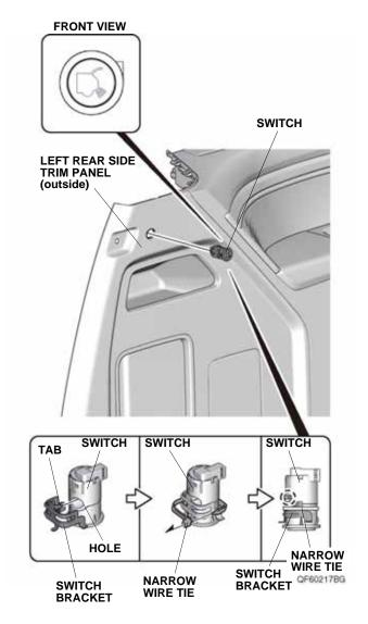
22. Line up the tab on the switch bracket with the hole on the switch and secure the switch bracket to the switch with one narrow wire tie.
