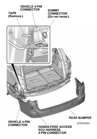
38. With the help of an assistant, bring the rear bumper close to the vehicle, and plug the Hands-Free Access ECU harness 4-pin connector into the vehicle 4-pin connector. Install the rear bumper. Go to step 43.
