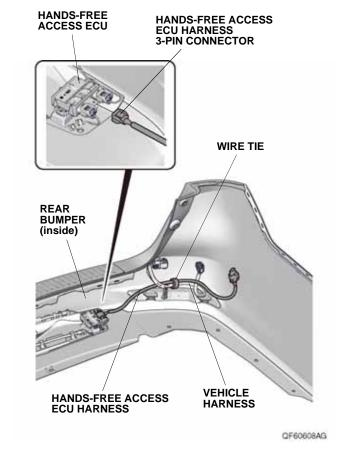
36. Secure the Hands-Free Access ECU harness to the vehicle harness with one wire tie.
