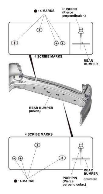
31. While wearing eye protection and drilling from the outside of the rear bumper, drill eight pierced marks with a 3 mm drill bit, then finish with a 6 mm drill bit. NOTE: Make sure to drill perpendicular to the rear bumper.
