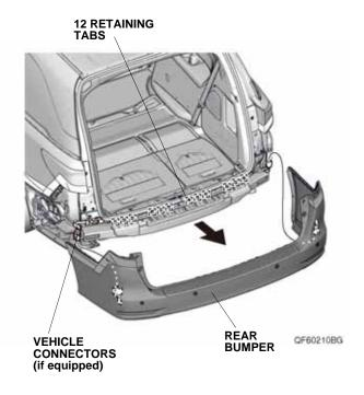
Remove the tapes to free the vehicle 2-pin connector, and unplug the vehicle 2-pin connector.
