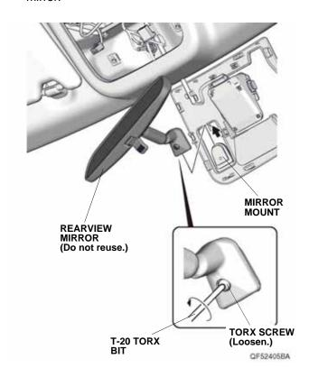
6. Install the automatic day/night mirror on the mirror mount as shown, and tighten the TORX screw.
