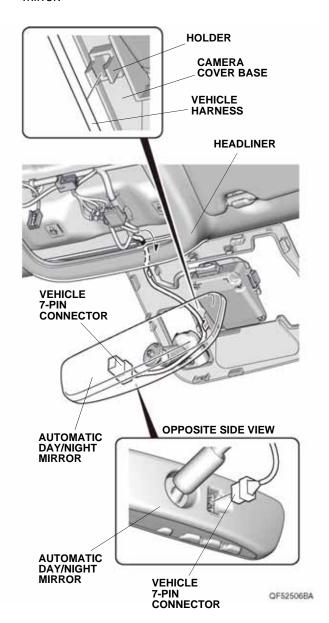
10. Using isopropyl alcohol on a shop towel, thoroughly clean the camera cover base where the aluminum tape will attach.
