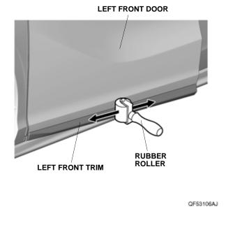
7. Line up and apply masking tape to the upper edge of the left front trim as shown.
