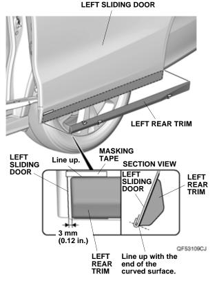
12. While applying light pressure against the left rear trim, carefully remove the taped adhesive backings.
