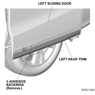
13. Secure the left rear trim to the left sliding door with two clips.
