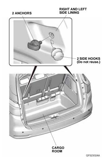
3. Install the cargo net onto the anchors and side hooks as shown.
