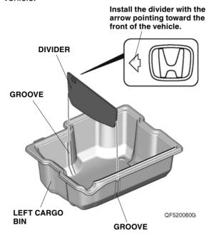
• To store the divider, snap it into the holders in the bottom of the left cargo bin.
