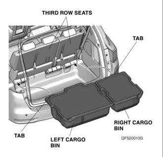
To stow either third row seat, remove the corresponding cargo bin and lid from the vehicle and lower the third row seat gently.
