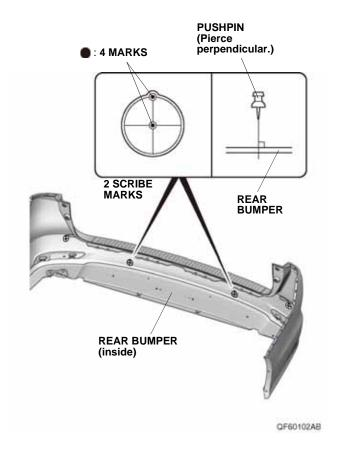
35. While wearing eye protection, drill the eight pierced marks with a 3 mm drill bit from the painted side of the rear bumper.
