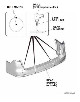
36. While wearing eye protection and drilling from painted side of the rear bumper, enlarge the left outer lower 3 mm hole and right outer lower 3 mm hole to 24 mm using a 24 mm hole saw.
