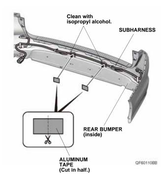
45. Using scissors, cut one piece of aluminum tape in half, and secure the subharness to the rear bumper with two halves of aluminum tape as shown.
