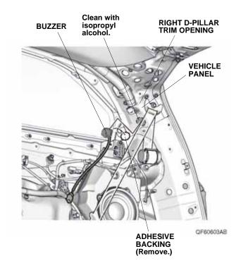
17. Remove the adhesive backing from the buzzer, and attach the buzzer to the vehicle panel as shown.
