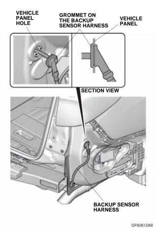
32. Install the connector clip on the backup sensor harness 8-pin connector, and secure the backup sensor harness 8-pin connector to the vehicle panel.
