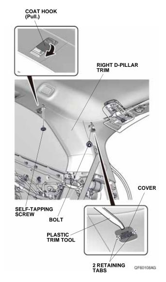
11. Using the plastic trim tool, open the cover and remove the bolt.
