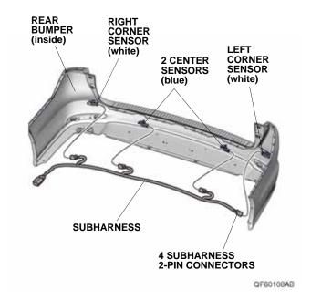
43. Secure the subharness to the rear bumper, left corner sensor clip, and two center sensor clips with three wire ties and two wire ties clip B as shown.
