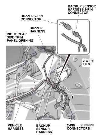
25. Secure the 2-pin connectors, backup sensor harness, and buzzer harness to the vehicle harness with two wire ties.
