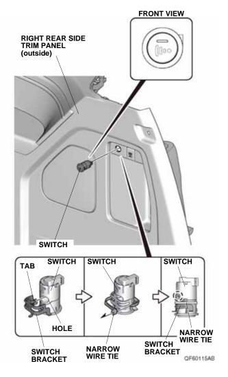
51. Line up the tab on the switch bracket with the hole on the switch and secure the switch bracket to the switch with one narrow wire tie.
