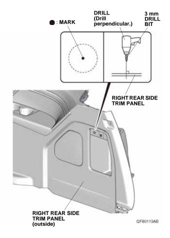
49. While wearing eye protection, enlarge the 3 mm hole to 26 mm using a 26 mm hole saw. Remove any burrs.
