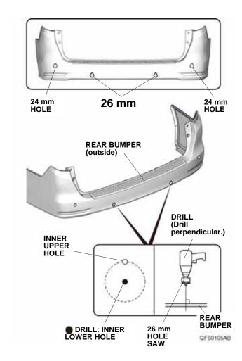
38. Insert the left corner sensor (white) and center sensor (blue) to the rear bumper.
