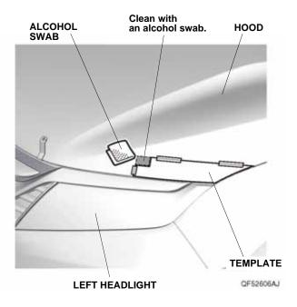
Remove the adhesive backing from the left bracket C, line it up with the template, and press the left bracket C against the hood to set the adhesive. Remove the template.
