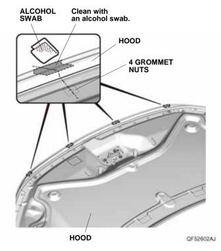
Remove the adhesive backings from the four protection films, and attach them to the front of the hood area where the two brackets A and the two brackets B will mount.
