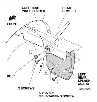
3. Remove one bolt and two screws from the right rear inner fender and rear bumper.
