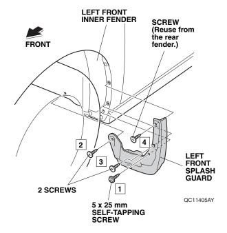
9. Turn the steering wheel fully clockwise, and repeat steps 6 through 8 to install the right front splash guard.
