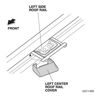
18. Install the left center roof rail cover to the left side roof rail as shown. Make sure that the left center roof rail cover is no clearance between the left side roof rail.
