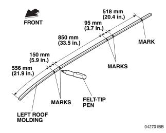
7. While wearing an eye protection, use an air saw to cut off the left roof molding at the mark made in step 6.
