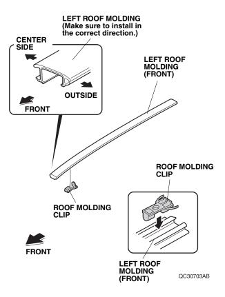
Reinstall the roof molding left cover.
