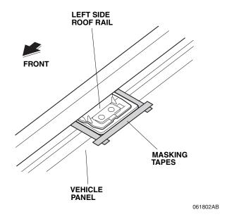
Hook the left center roof rail cover to the left side roof rail as shown.
