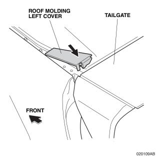
10. Reinstall the left roof moldings back onto the roof of the vehicle as shown.
