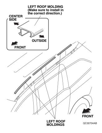
Install the left side roof rail with six Torx nuts. Make sure the roof rail is installed in the correct position.
