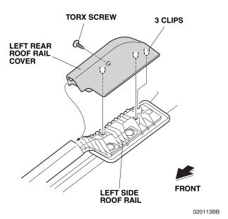
15. Secure the left rear roof rail cover to the left side roof rail with one Torx screw.
