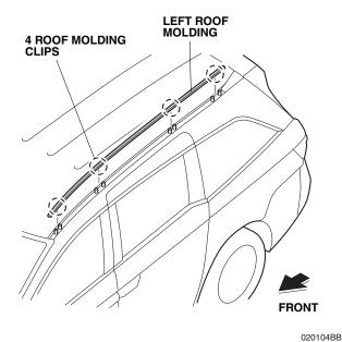
2. Open the tailgate halfway. Using a trim tool, pry up on the rear end of the roof molding left cover.
