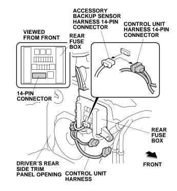
19. Plug the accessory backup sensor harness 14-pin connector into the control unit harness 14-pin connector.
