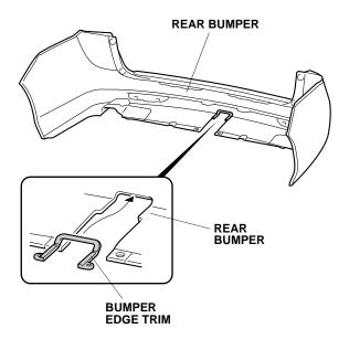
36. Using a felt-tip pen, mark the centers of the bumper edge trim holes.
