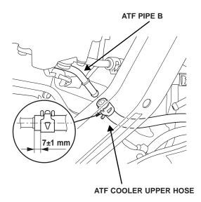
Touring: Remove the plug from the ATF filter, and connect the ATF cooler upper hose. Install the hose clamp. Align the paint marks as shown.
