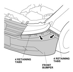
• Remove four self-tapping screws, eight bolts, and the four clips from the front bumper.
