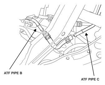
Touring: Remove the hose that connects the ATF filter and ATF pipe C, and put plugs in both the ATF filter and ATF pipe C to prevent leaks.
