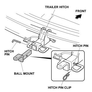
After the first 600 miles (1,000 km) of towing, have your Honda Dealer re-check the tightness of the trailer hitch bolts.
