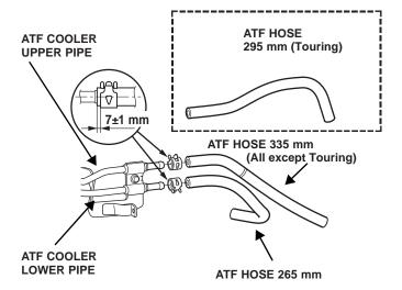
61. Route the hoses installed on the ATF cooler through the hole cut in the left air guide, and fit the ATF cooler into place on the bulkhead. Install the three washerbolts from the kit through the ATF cooler into the threaded holes in the front bulkhead. Tighten the bolts securely.
