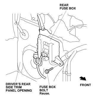
23. Install the control unit to the vehicle panel with the fuse box bolt removed step in 22.
