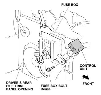
24. Plug the control unit harness 12-pin connector into the control unit.
