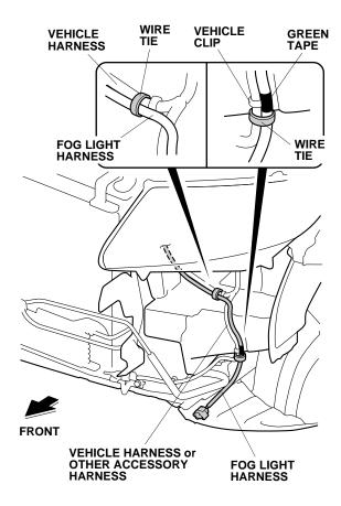
22. Secure the fog light harness to the vehicle harness with one wire tie. Go to step 25.
