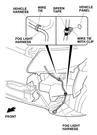
24. Secure the fog light harness to the vehicle harness with one wire tie.
