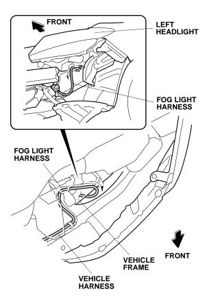
If the vehicle is equipped with a vehicle harness or another accessory harness, continue with step 21. If not, go to step 23.
