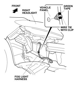
18. Secure the fog light harness to the vehicle harness with two wire ties.
