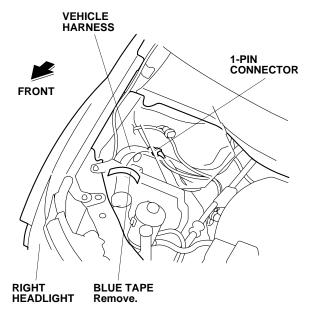
13. Plug the fog light harness 1-pin connector to the vehicle 1-pin connector.
