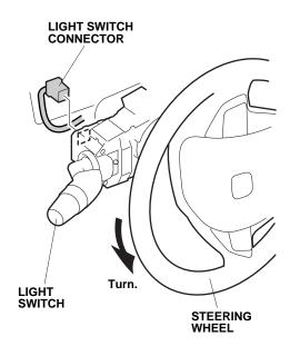
34. Remove two self-tapping screws from the light switch. While pushing the retaining tab, slide the light switch out, and remove it from the steering column. Do not pull on the lever when removing the case, or damage the tab hole in the steering column.
