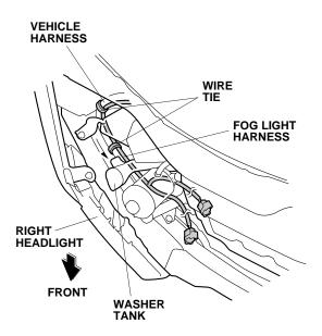
16. Continute routing the fog light harness under the right headlight as shown.
