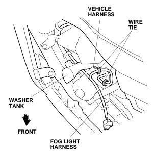
19. Route the fog light harness along the vehicle harness, and secure it to the vehicle harness with six wire ties.
