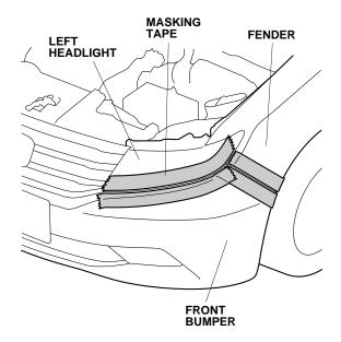
Release eight retaining tabs on each side of the front bumper.
