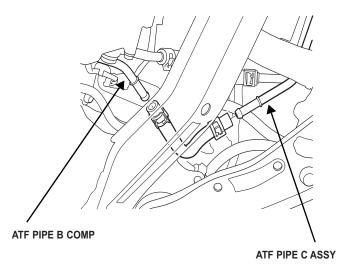
6AT: Remove the hose that connects the ATF filter and ATF pipe C assy, and put plugs in both ATF filter and ATF pipe C assy to prevent leaks.
