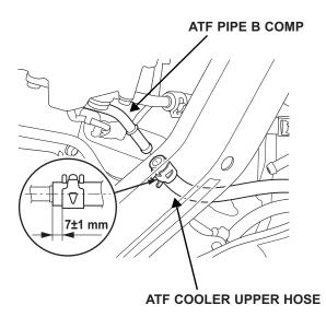
6AT: Remove the plug from the ATF filter, and connect the ATF cooler upper hose. Install the hose clamp. Align the paint marks as shown.
