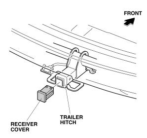
Install the ball mount the trailer hitch using a hitch pin clip and hitch pin.
