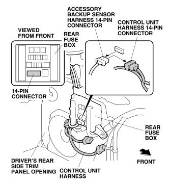
Plug the accessory backup sensor harness 14-pin connector into the control unit harness 14-pin connector.
