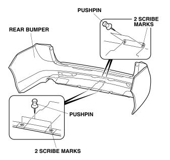
32. While wearing eye protection, drill the front two pierced marks of the rear bumper. First drill with a 3 mm drill bit, and finish with a 10 mm drill bit. Remove any burrs.
