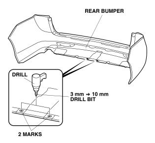
33. Drill the rear two pierced marks of the rear bumper. First drill with a 3 mm drill bit, and finish with a 10 mm drill bit.
