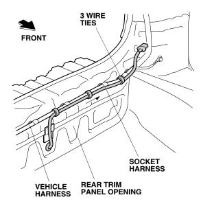
14. Get the control unit harness. Plug the control unit harness 4-pin connector to the socket harness 4-pin connector.
