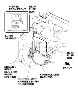
21. Insert the control unit onto the control unit bracket.
