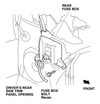
23. Install the control unit to the vehicle panel with the fuse box bolt removed in step 22.
