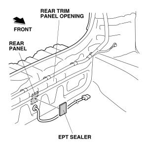
12. Attach the EPT sealer to the rear panel as shown.
