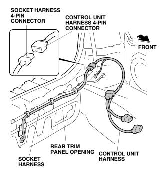
15. Remove one vehicle ground bolt from the vehicle ground terminal.
