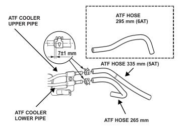
61. Route the hoses installed on the ATF cooler through the hole cut in the left air guide, and fit the ATF cooler into place on the bulkhead. Install the three washerbolts from the kit through the ATF cooler into the threaded holes into the front bulkhead. Tighten the bolts securely.
