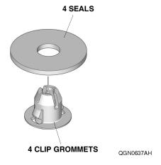
Install the four clip grommets to the four 8.5 mm holes on the trunk lid as shown.
