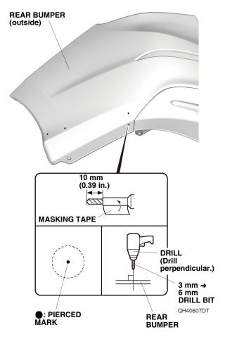
4. Using a file, remove any burrs from the hole.
