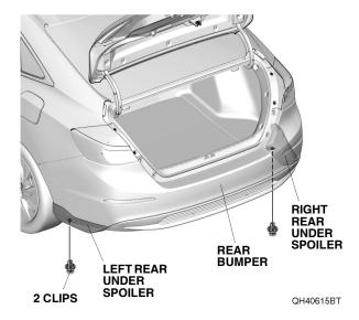
18. Secure the left and right rear under spoilers to the rear bumper.
