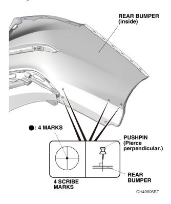
3. While wearing eye protection, drill the pierced mark to 6 mm as shown.
