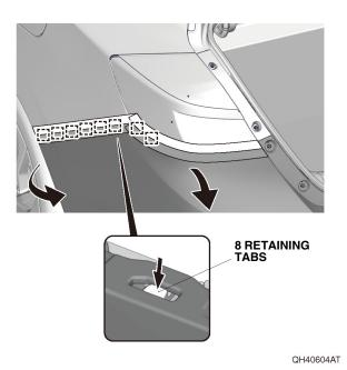
With the help of an assistant, remove the rear bumper. Place the rear bumper on a blanket to prevent damage.
