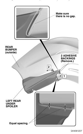
13. Tighten the one self-tapping screw loosely installed in step 10.
