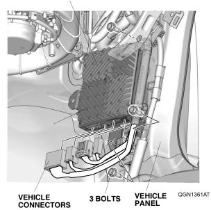
38. Unplug the vehicle connector, and release the vehicle harness as shown.
