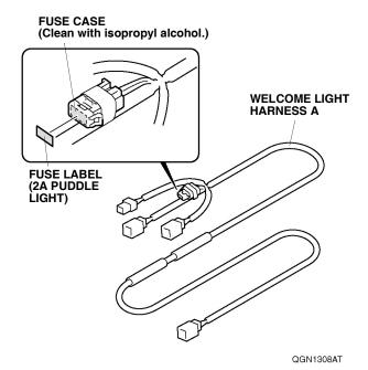
23. Attach the fuse label to the welcome light harness A fuse case.
