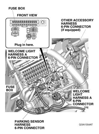
27. Attach the welcome light harness A 6-pin connector (white) to any of the positions shown. Go to step 30.
