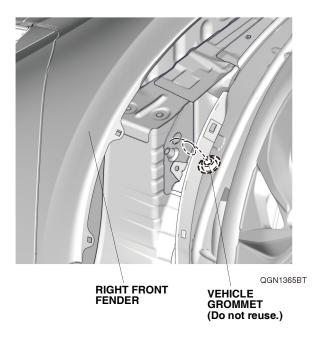
41. Route the subharness through the vehicle panel hole, and secure the subharness grommet to the vehicle panel.
