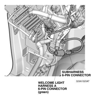
53. Secure the 6-pin connectors and subharness to the vehicle harness with two wire ties. Go to step 57.
