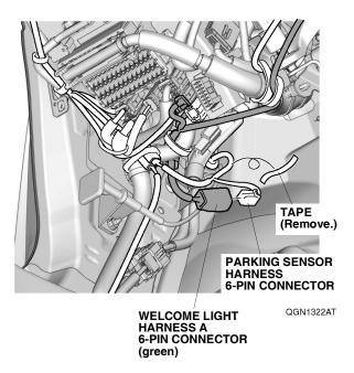
56. Secure the 6-pin connectors to the vehicle harness with one wire tie.
