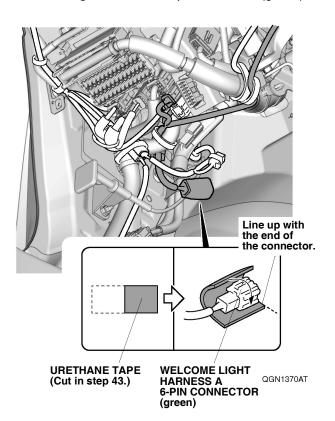
55. Remove the tape from the parking sensor harness, and plug the parking sensor harness 6-pin connector into the welcome light harness A 6-pin connector (green).
