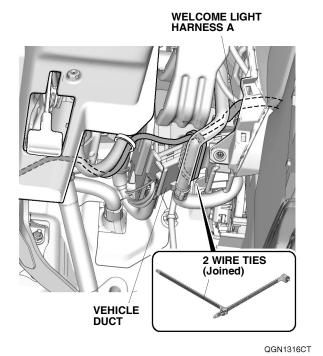
36. Route welcome light harness A as shown, and secure it to the vehicle harness with four wire ties.
