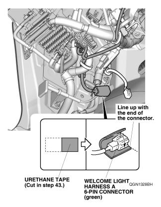
52. Plug the subharness 6-pin connector into the welcome light harness A 6-pin connector (green).
