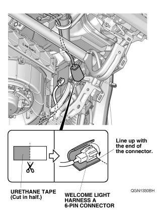
44. Plug the subharness 6-pin connector into the welcome light harness A 6-pin connector.
