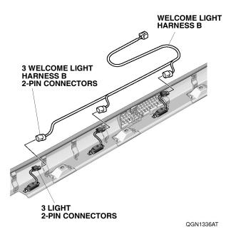
66. Install the two wire ties to the 2-pin connectors, and secure the 2-pin connectors to the left side sill trim with two wire ties as shown.
