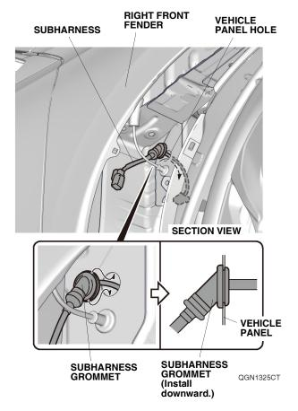
42. Install the amplifier (with amplifier only) and vehicle harness, then plug in the vehicle connectors removed in steps 37 and 38.
