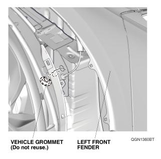
49. Route the subharness through the vehicle panel hole, and secure the subharness grommet to the vehicle panel.
