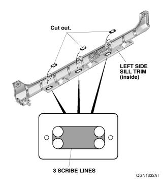
62. Install the six spring nuts on the left side sill trim. NOTE: Make sure to install the spring nut in the correct orientation.
