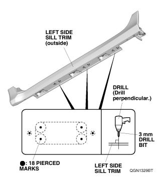
59. While wearing eye protection, enlarge the 3 mm holes on the left side sill trim with a 6 mm drill bit. Remove any burrs.
