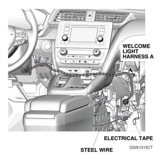
35. Join two wire ties together as shown, then secure welcome light harness A to the vehicle duct with one joined wire ties.
