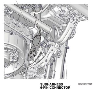
45. Secure the 6-pin connectors to the vehicle harness with one wire tie.
