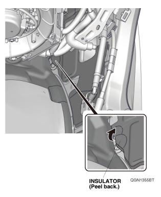
40. Remove the vehicle grommet as shown.
