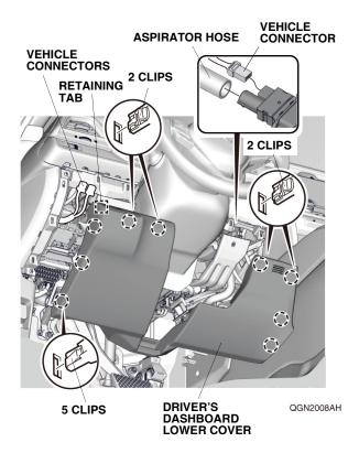
9. Pull away the door opening seal, and remove the driver's dashboard side lid.
