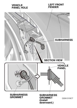
50. Install the vehicle harness released in step 46.
