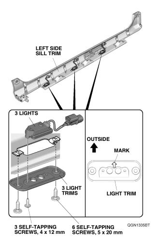
65. Plug the welcome light harness B 2-pin connectors into the light 2-pin connectors.
