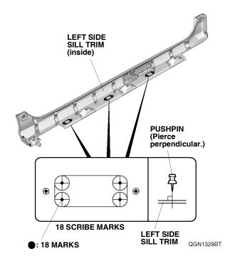
58. While wearing eye protection, drill the 18 pierced marks on the left side sill trim with a 3 mm drill bit. NOTE: Make sure to drill perpendicular to the left side sill trim.
