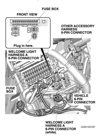
29. Attach the 6-pin connectors to any of the positions shown.
