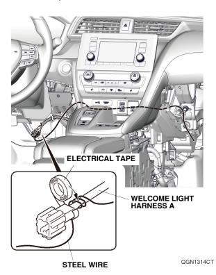
34. Route welcome light harness A as shown, and remove the electrical tape and steel wire.
