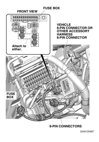
30. Line up the branch of welcome light harness A with the branch of the vehicle harness, and secure it to the vehicle harness with one wire tie as shown.
