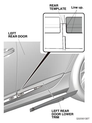
13. While applying light pressure against the left rear door lower trim, carefully remove the taped adhesive backings.
