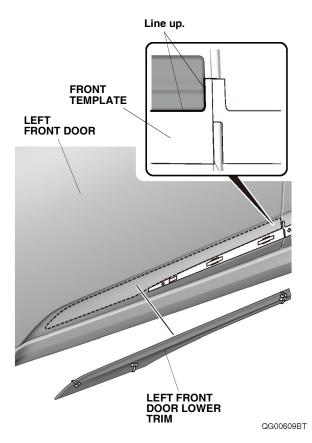
9. While applying light pressure against the left front door lower trim, carefully remove the taped adhesive backings.
