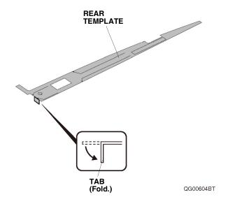
4. Line up the bottom of the rear template with the curved end. Then, line up the front of the rear template with the edge of the left rear door, and attach it to the left rear door with masking tape as shown.
