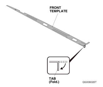
Line up the bottom of the front template with the curved end. Then, line up the rear of the front template with the edge of the left front door, and attach it to the left front door with masking tape as shown.
