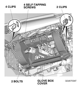
6. Remove the driver's dashboard lower cover, and unplug the vehicle connectors.
