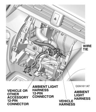
26. Secure the clip on the ambient light harness to the vehicle panel.
