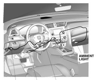
2 FUSES, 2A AMBIENT AMBIENT LIGHT QGN1601AT LIGHT HARNESS
