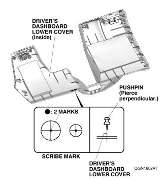
11. While wearing eye protection, drill the pierced mark on the driver's dashboard lower cover to 5 mm. First, drill with a 3 mm drill bit, then finish with a 5 mm drill bit.
