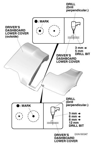
12. While wearing eye protection, drill the pierced mark on the driver's dashboard lower cover to 12 mm. First, drill with a 3 mm drill bit, next, with a 6 mm drill bit, then with an 8 mm drill bit, and finish with a 12 mm drill bit.
