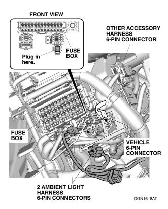
34. Attach the 6-pin connectors to any of the positions shown.
