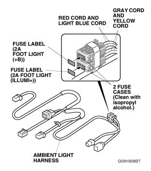
22. Apply the fuse labels to the ambient light harness fuse cases.
