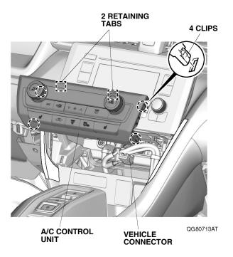
Remove the audio unit, and unplug the vehicle connectors.
