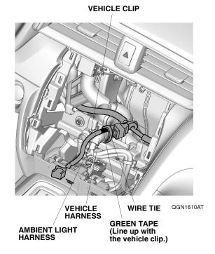
25. Plug the vehicle or other accessory 12-pin connector into the ambient light harness 12-pin connector, and secure it to the vehicle harness with one wire tie.
