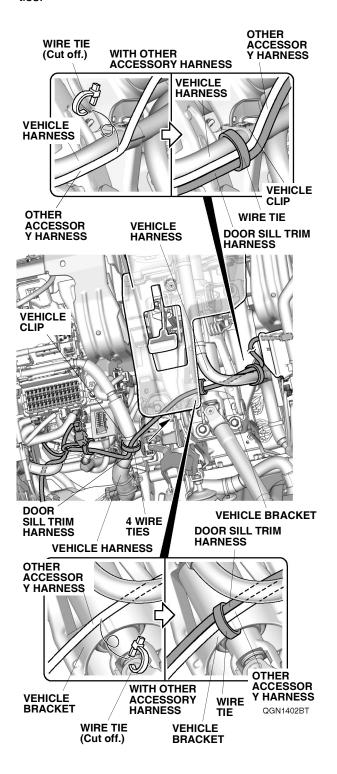
21. Secure the door sill trim harness to the vehicle duct with the two wire ties.
