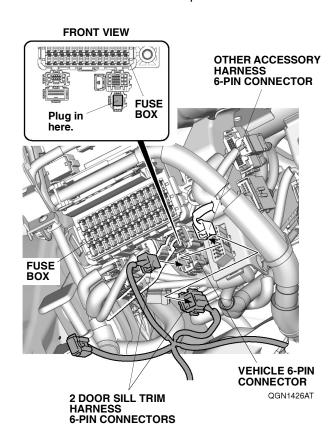
18. Attach the 6-pin connectors to any of the positions shown.
