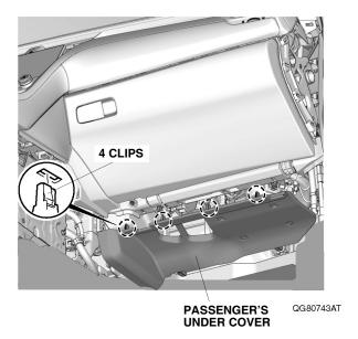
6. Open the glove box, push inward on the glove box stops, and remove the glove box.
