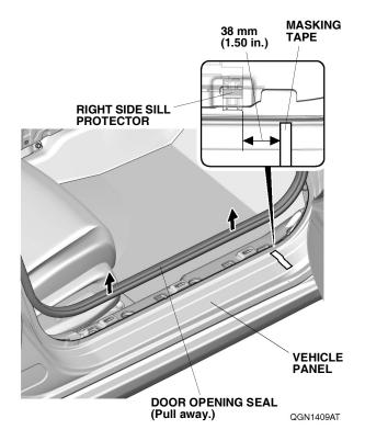
27. Peel back the ends of two adhesive backings on the right door sill trim, and attach them to the front of the trim with masking tape.
