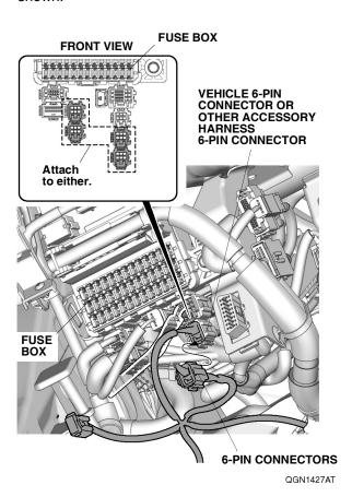
19. Attach the door sill trim harness fuse case to the vehicle connector.
