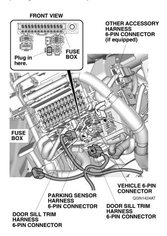
16. Attach the door sill trim harness 6-pin connector to any of the positions shown. Go to step 19.
