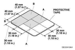
26. Pull away the door opening seal, and apply masking tape to the vehicle panel as shown.
