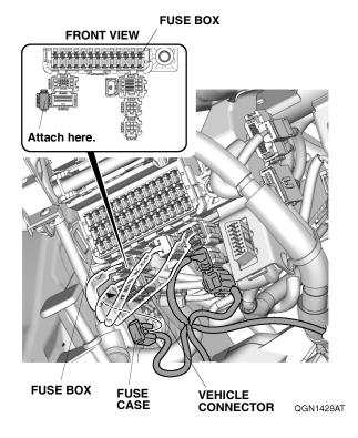
20. Route the door sill trim harness as shown. Secure it to the vehicle harness and bracket with the four wire ties.
