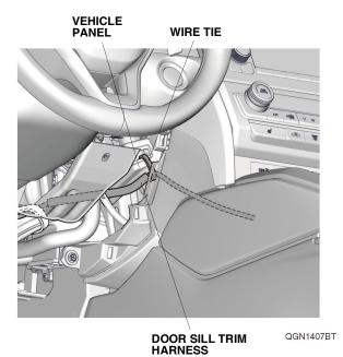
24. Route the door sill trim harness as shown. Secure the door sill trim harness to the vehicle harness with the four wire ties.
