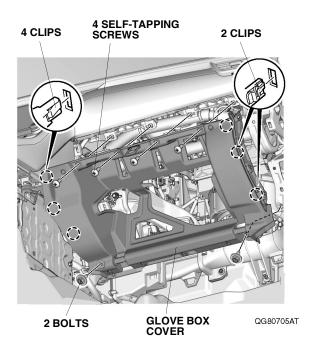
8. Remove the driver's dashboard lower cover, and unplug the vehicle connectors.
