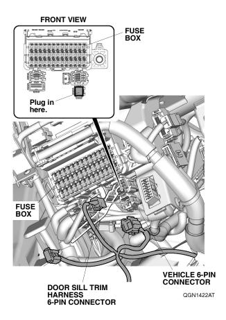
14. Attach the door sill trim harness 6-pin connector to the vehicle 6-pin connector. Go to step 19.
