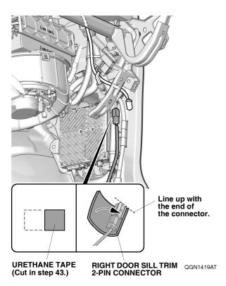
48. Plug the door sill trim harness 2-pin connector into the right door sill trim 2-pin connector.
