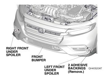
17. Remove the two adhesive backings. Press the right front under spoiler and left front under spoiler firmly against the front bumper with the palm of your hands.
