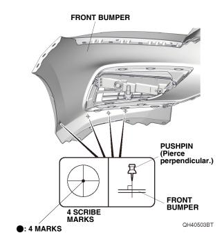
5. While wearing eye protection, drill the two pierced marks to 6 mm.
