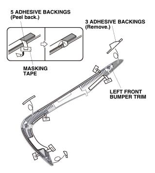
8. Line up the left front bumper trim with the front bumper as shown. Loosely install the left front bumper trim to the front bumper with three self-tapping screws and three washers.
