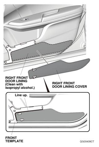
4. Line up the right front door lining cover with the front template, and attach it as shown.
