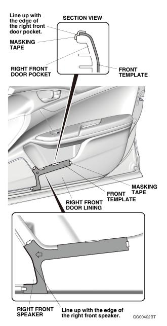
Peel back the adhesive backings, and tape them to the front surface of the right front door lining cover with masking tape. Remove the remaining adhesive backings.
