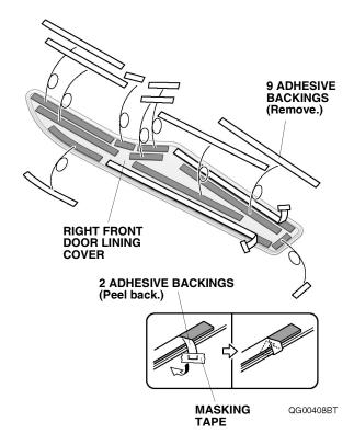
3. Using isopropyl alcohol on a shop towel, thoroughly clean the area where the right front door lining cover will attach.
