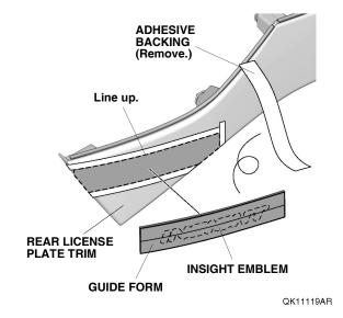
Remove the guide form and using the palm of your hand, firmly press the INSIGHT emblem against the rear license plate trim for 30 seconds.
