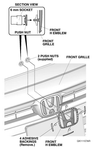
11. Using the palm of your hand, firmly press the front H emblem against the front grille for 30 seconds.
