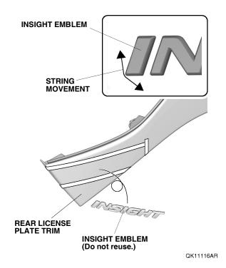
21. Install the INSIGHT emblem in the guide form, and temporarily secure it with masking tape.
