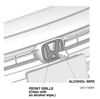
10. Remove the four adhesive backings from the front H emblem. Install the front H emblem to the front grille as shown.
