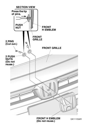
9. Using an alcohol wipe, thoroughly clean the front grille where the front H emblem will attach.
