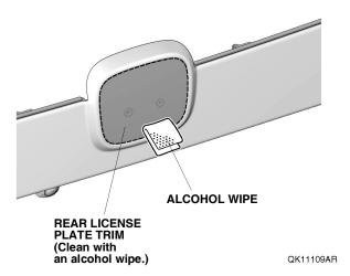
14. Remove the four adhesive backings from the rear H emblem. Install the rear H emblem to the rear license plate trim as shown.
