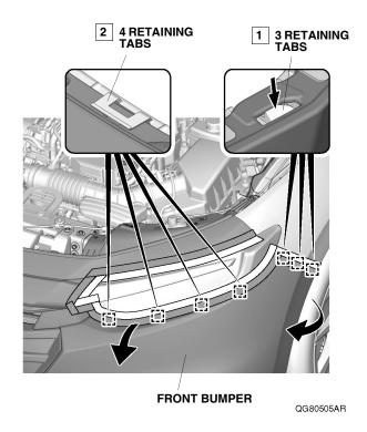
With the help of an assistant, remove the front bumper, and unplug the vehicle connectors (if equipped). Place the front bumper on a blanket to prevent damage.
