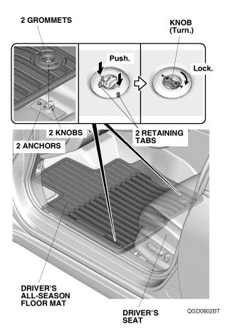
2. Place the grommets in the driver's all-season floor mat over the anchors. Push the grommets into the anchors to secure the retaining tabs, then turn the knobs 90° to secure the driver's all-season floor mat.
