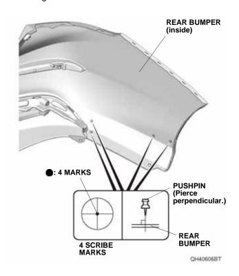
3. While wearing eye protection, drill the pierced mark to 6 mm as shown.
