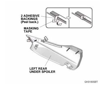
10. Loosely install the left rear under spoiler to the rear bumper with one self-tapping screw and clip A.
