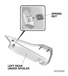
Peel back the adhesive backings, and tape them to the front surface of the left rear under spoiler with masking tape.
