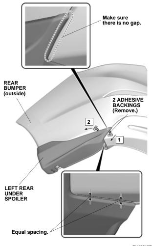
13. Tighten the one self-tapping screw loosely installed in step 10.
