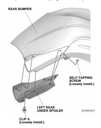
11. Loosely install the three female clips into each male clip as shown.
