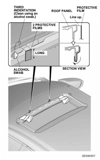
7. Remove the adhesive backing from the two protective films, and attach them to the roof panel at the third indentation.
