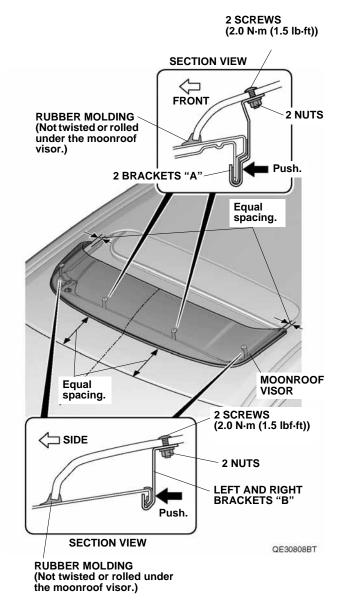
14. Tighten two screws and two nuts on the front of the vehicle first, then tighten two screws and two nuts on each side. Tighten while applying pressure so that there is no gap between the roof panel and the brackets "A" and "B". Torque the screws to 2.0 N·m (1.5 lb·ft).
