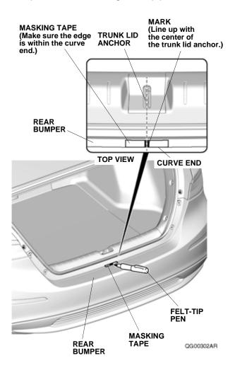
2. Line up the sticker on the rear bumper metal panel with the mark on the masking tape. Then, attach masking tape at both ends as shown.
