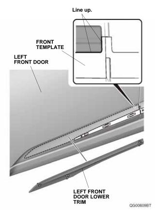
9. While applying light pressure against the left front door lower trim, carefully remove the taped adhesive backings.
