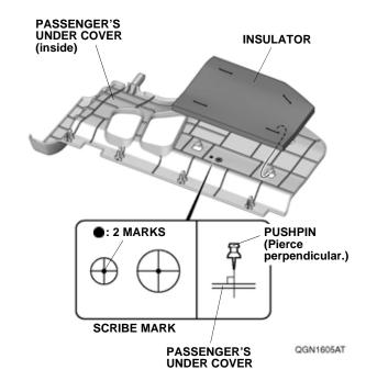
16. While wearing eye protection, drill the pierced mark on the passenger's under cover to 5 mm. First, drill with a 3 mm drill bit, then finish with a 5 mm drill bit. NOTE: Drill perpendicular to the passenger's under cover.
