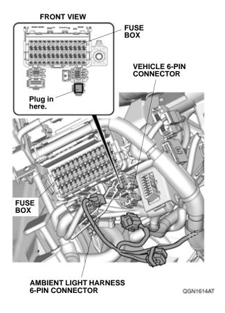
30. Attach the ambient light harness 6-pin connector to the vehicle 6-pin connector. Go to step 35.
