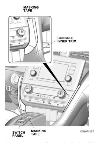
8. Remove the A/C control unit, and unplug the vehicle connector.
