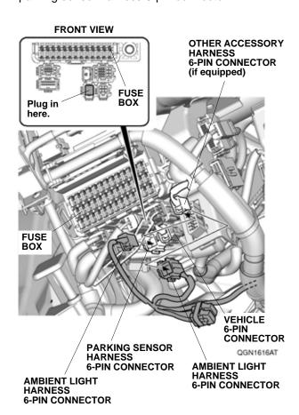
32. Attach the ambient light harness 6-pin connector to any of the positions shown. Go to step 35.
