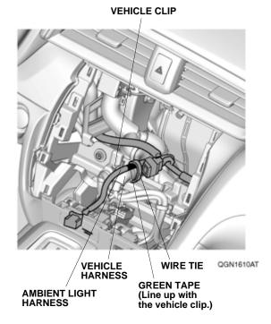
25. Plug the vehicle or other accessory 12-pin connector into the ambient light harness 12-pin connector, and secure it to the vehicle harness with one wire tie.
