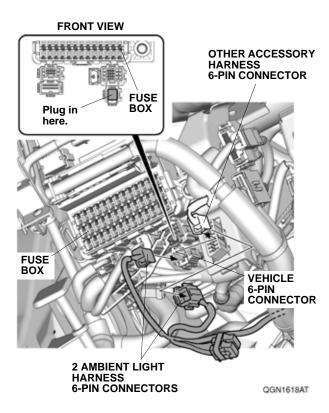
34. Attach the 6-pin connectors to any of the positions shown.
