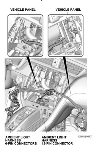
24. Line up the green tape on the ambient light harness with the vehicle clip, and secure the ambient light harness to the vehicle harness with one wire tie.
