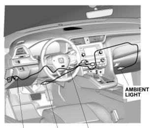
2 FUSES, 2A AMBIENT AMBIENT LIGHT QGN1601AT LIGHT HARNESS
