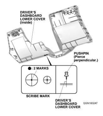
11. While wearing eye protection, drill the pierced mark on the driver's dashboard lower cover to 5 mm. First, drill with a 3 mm drill bit, then finish with a 5 mm drill bit.
