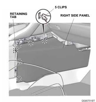
2. Pull away the door opening seal, and remove the passenger's dashboard side lid.
