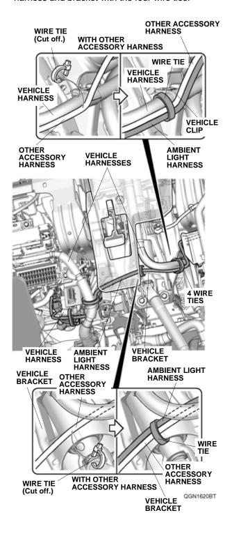
36. Secure the ambient light harness to the vehicle duct with the two wire ties.
