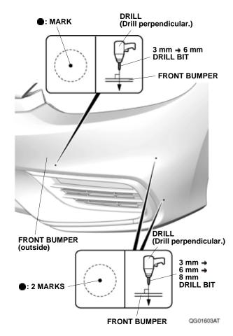
5. While wearing eye protection, enlarge the two 6 mm outer holes to 8 mm with an 8 mm drill bit. Remove any burrs.
