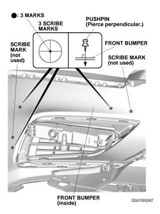
4. While wearing eye protection, drill the three pierced marks on the front bumper to 6 mm. First, drill with a 3 mm drill bit, then finish with a 6 mm drill bit.
