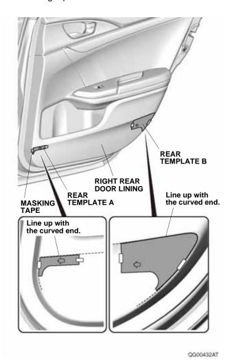
11. Peel back the adhesive backings, and tape them to the front surface of the right rear door lining cover with masking tape. Remove the remaining adhesive backings.
