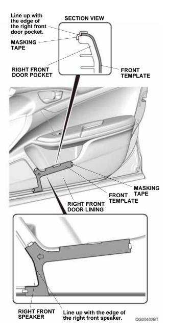
Peel back the adhesive backings, and tape them to the front surface of the right front door lining cover with masking tape. Remove the remaining adhesive backings.
