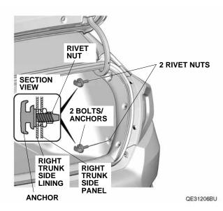
14. Install the cargo net on the anchors in the trunk.
