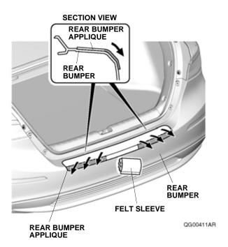
12. Using a shop towel, wipe up the 3M protective tape application solution. Allow the rear bumper applique to dry thoroughly.
