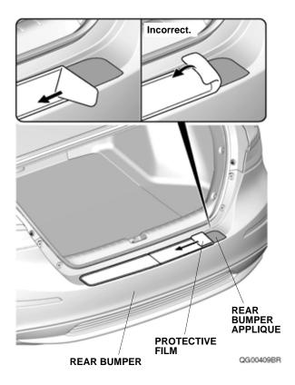
Repeat step 7 at the center of the lower section on the rear bumper applique.
