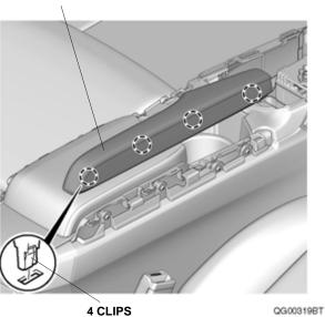
18. Remove the console rear panel, and unplug the vehicle connectors.
