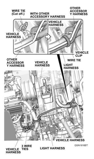
45. Secure the light harness to the vehicle duct with the two wire ties.
