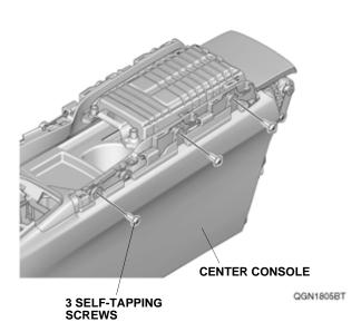
29. Route the left light harness inside the center console, and install the left light with the three self-tapping screws while pushing up the left light.
