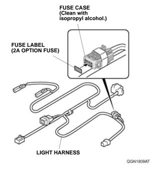
36. Apply the fuse label to the light harness fuse case.
