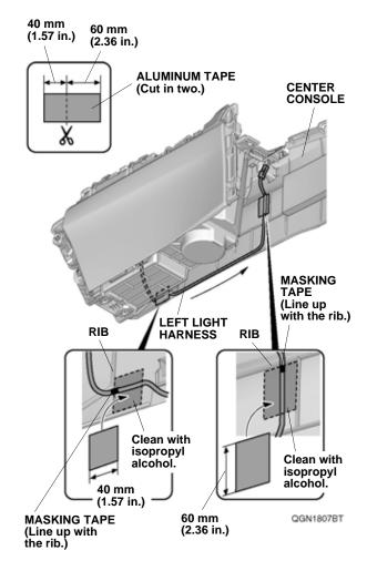
31. Using scissors, cut one piece of aluminum tape as shown. Secure the left light harness to the center console with two pieces of aluminum tape.
