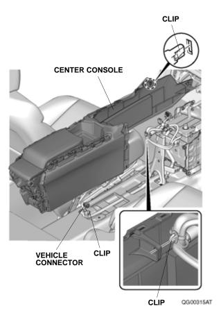
20. Remove the driver's dashboard lower cover, and unplug the vehicle connectors.
