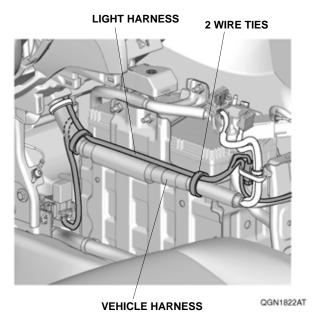
54. Plug the left and right light 2-pin connectors into the light harness 2-pin connectors, and install the center console.
