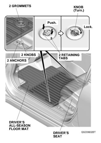
2. Place the grommets in the driver's all-season floor mat over the anchors. Push the grommets into the anchors to secure the retaining tabs, then turn the knobs 90° to secure the driver's all-season floor mat. 3. Install the passenger's all-season floor mat as shown.
