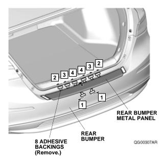
8. Using a rubber roller, apply firm pressure against the rear bumper metal panel and roll from the center to the outside.
