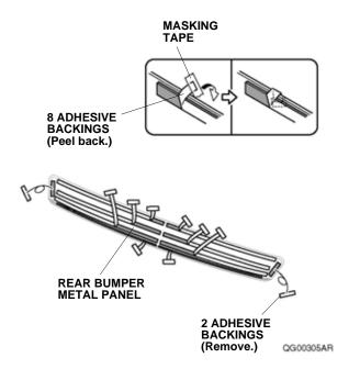
6. Attach the rear bumper metal panel to the rear bumper by lining it up with the masking tape as shown.
