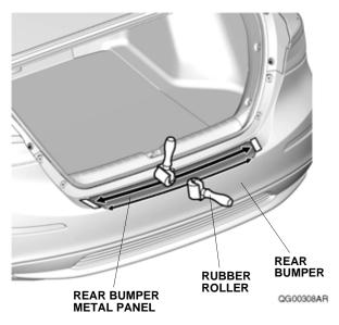
9. Remove masking tape and the sticker on the rear bumper metal panel.
