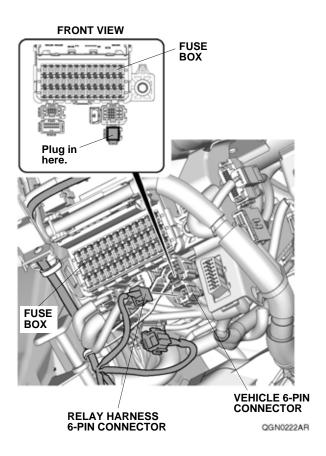
38. Attach the relay harness 6-pin connector to the vehicle 6-pin connector. Go to step 43.
