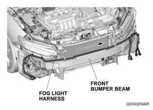
23. Route the fog light harness as shown. Attach the two fog light harness ground terminals with the ground bolt provided.
