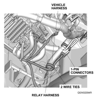
45. Attach the wire tie with holder to the relay harness relay block, and secure it to the vehicle harness with the wire tie with holder.
