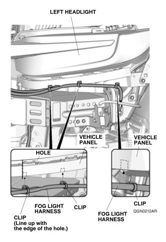
26. Join four long wire ties together as shown, and secure the fog light harness to the front bumper beam with those wire ties.
