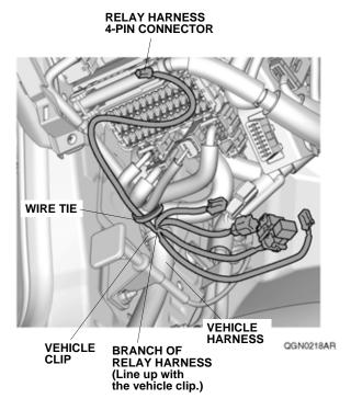
If the vehicle is equipped with another accessory harness 4-pin connector, go to step 35; otherwise, continue with step 34.
