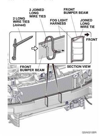
27. Join eight long wire ties together as shown, and secure the fog light harness to the front bumper beam with those wire ties.
