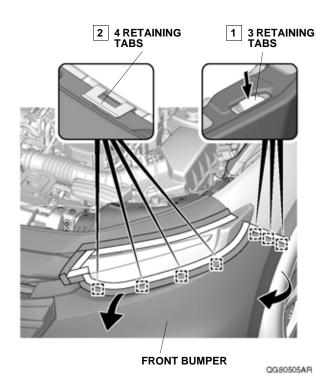
With the help of an assistant, remove the front bumper using a plastic trim tool. Place the front bumper on a blanket to prevent damage.
