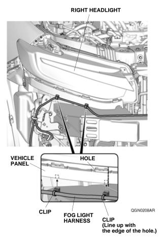
22. Route the fog light harness along the front bumper beam as shown.
