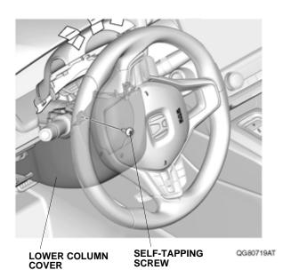
10. Turn the steering wheel 180° clockwise, and remove the self-tapping screw from the lower column cover.
