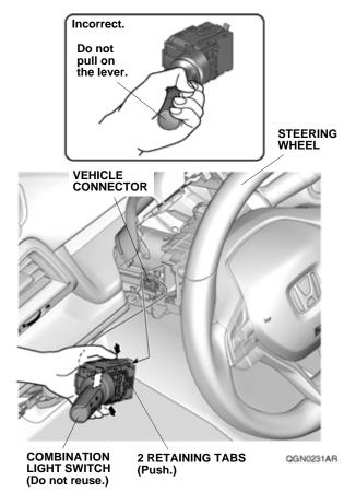
47. While pushing the two retaining tabs, slide the combination light switch out and remove it from the steering column.
