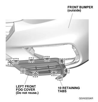
15. Install the left fog light trim to the front bumper with 10 retaining tabs.
