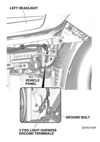
24. Route the fog light harness as shown. Line up the green tape on the fog light harness with the vehicle wire tie, and secure the fog light harness to the vehicle harness with one wire tie.
