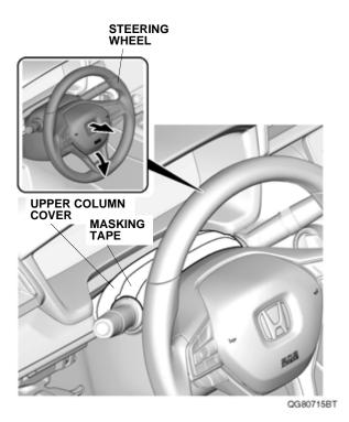
6. Turn the steering wheel 90° clockwise. Using a plastic trim tool, release the two hooks.
