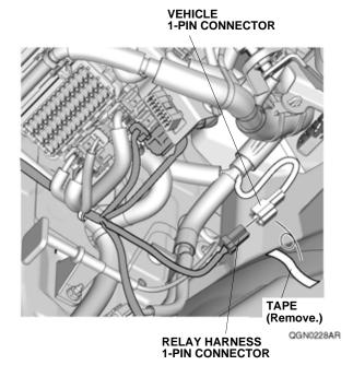
44. Secure the 1-pin connectors and relay harness to the vehicle harness with two wire ties.
