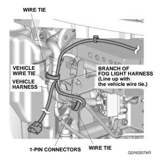
21. Secure the two clips on the fog light harness to the vehicle panel as shown.
