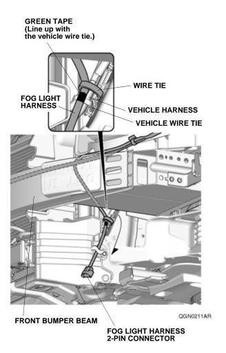
25. Secure the three clips on the fog light harness to the vehicle panel as shown.
