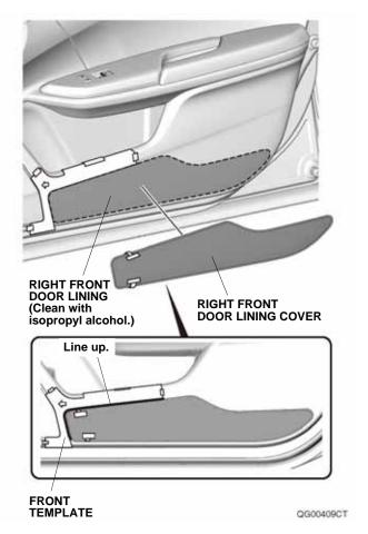
4. Line up the right front door lining cover with the front template, and attach it as shown.
