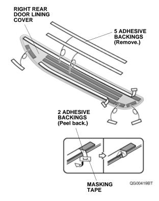
12. Using isopropyl alcohol on a shop towel, thoroughly clean the area where the right rear door lining cover will attach.
