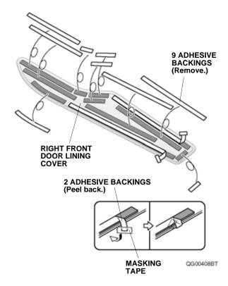
Using isopropyl alcohol on a shop towel, thoroughly clean the area where the right front door lining cover will attach.
