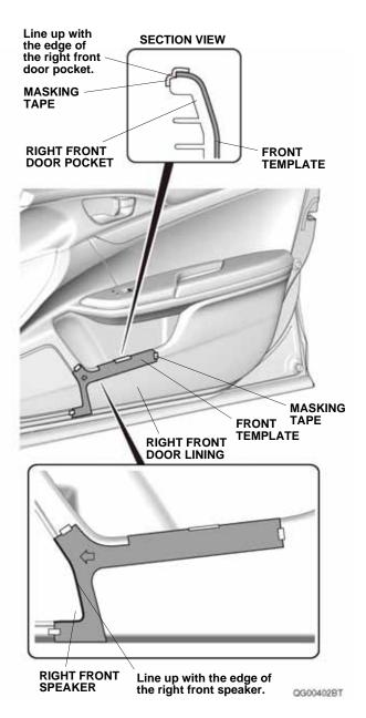
2. Peel back the adhesive backings, and tape them to the front surface of the right front door lining cover with masking tape. Remove the remaining adhesive backings.
