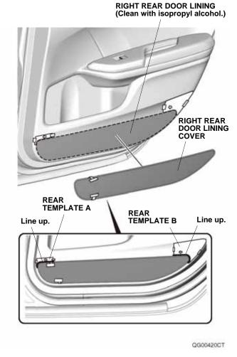
13. Line up the right rear door lining cover with rear templates A and B, attach it as shown.
