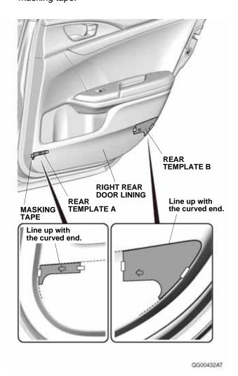
Peel back the adhesive backings, and tape them to the front surface of the right rear door lining cover with masking tape. Remove the remaining adhesive backings.
